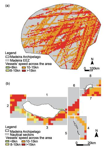
Fig. 4. Speed grid cell maps displayed within the Madeira ZEE area. Each pixel represents the vessels Speed Over Ground (SOG) average value. Only one representative map (July 2008) is displayed among the 20 representative months used in the present study. The 'low' speed cells are coloured in green and yellow and the 'high' speed cells are coloured in orange and red: (a) offshore traffic; (b) inshore traffic.
