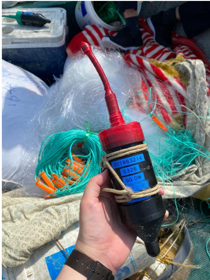
Figure 5. A SoundTrap ST300HF prepared for deployment on active gillnets on Cheung Chau, Hong Kong.
