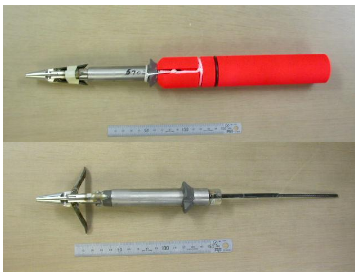
Fig. 3. The satellite tag used in this study. Upper photograph indicates the tag with a retrievable float at firing. Lower photograph indicates the tag without the float.
