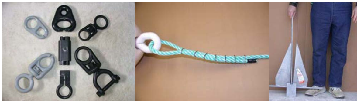
Figure 11. Gear modifications for fixed gear as part of the ALWTRP on the U.S. east coast to reduce whale entanglements: weak links and modified anchors.
