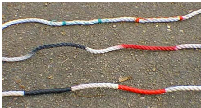
Figure 12. Gear marking strategies as part of the ALWTRP on the U.S. east coast to help identify gear type
