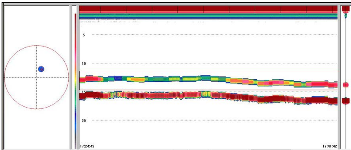
Figure A1. Transducer calibration process. The left window shows all the transducer quadrants with the position of the sphere in the beam; the sphere was located on the starboard forward quadrant at the time of saving this window. The right window, the top track is the calibration sphere echo and the bottom track is the echo of the suspended weight.
