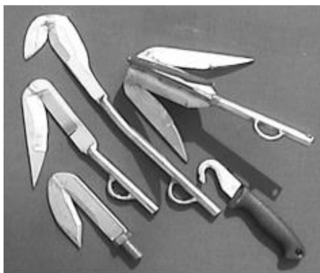
Fig. 3. Knives and other cutting tools used in disentanglement. Photo: Center for Coastal Studies, http://www.coastalstudies.org .
