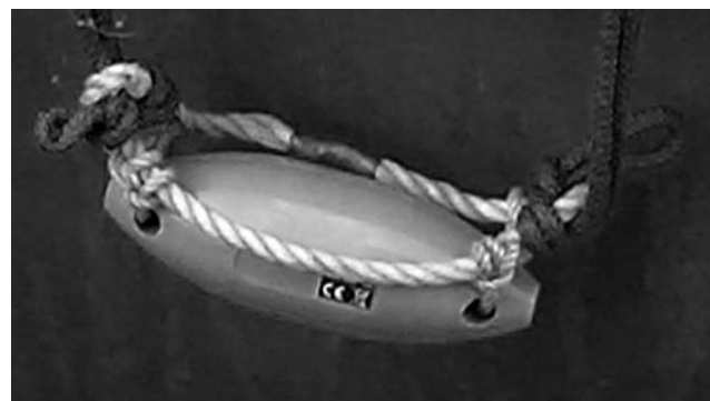
Fig. 2. Pinger attached to foot rope of static netting.
