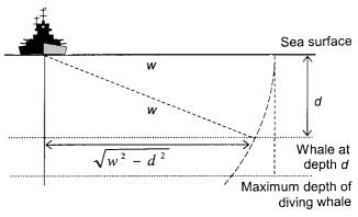
Fig. 5. Cross section view of volume of water surveyed (w = estimated strip half-width).
