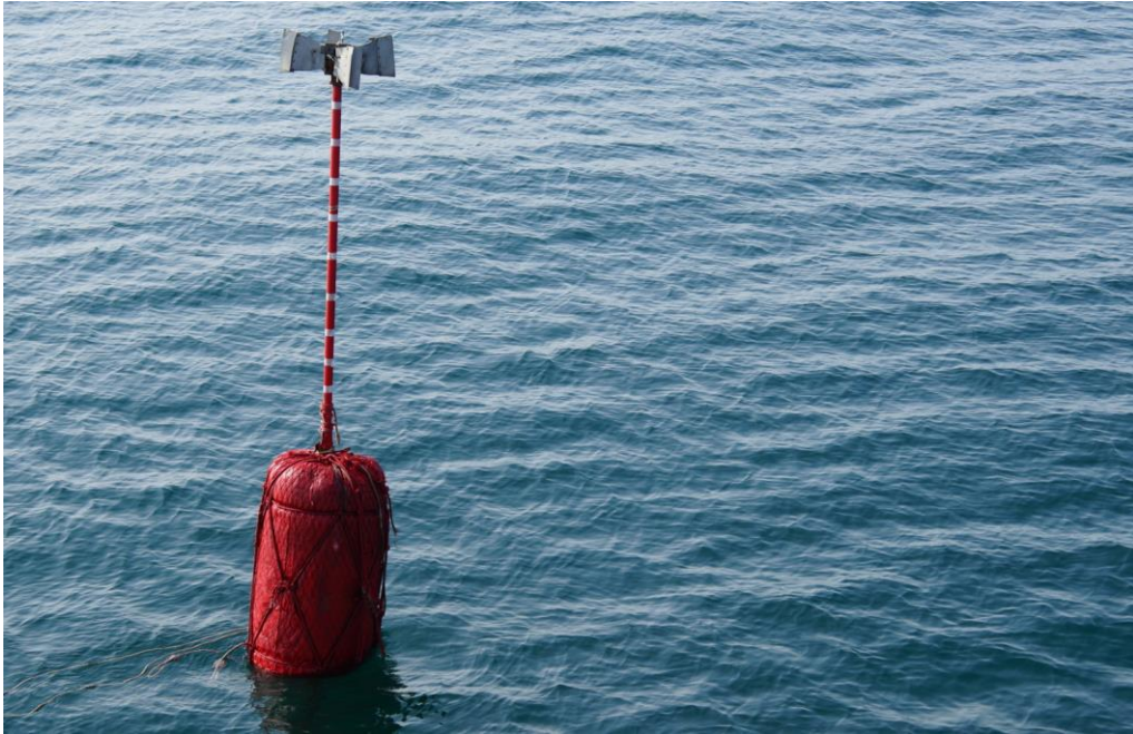
Figure 5. Radar reflecting buoy for estimated angle and distance training and experiment
