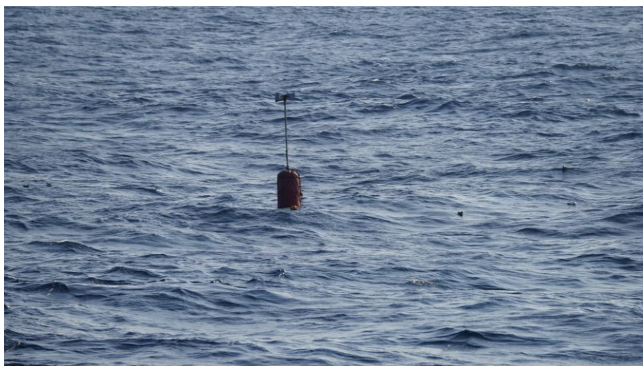
Figure 5. Radar reflecting buoy for estimated angle and distance training and experiment
