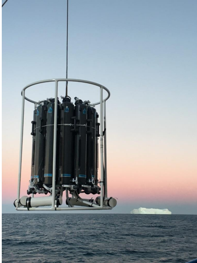
Figure 4.6.1: CTD deployment © Lavenia Ratnarajah, University of Liverpool
