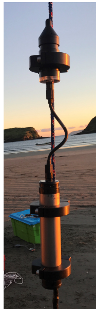
Figure 2 – Hidrophone system (Hydrophone Soundtrap STD 300, battery pack and frame)
