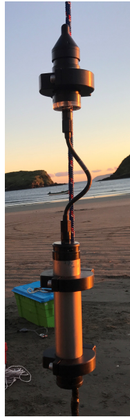
Figure 2 – Hydrophone system (Hydrophone Soundtrap STD 300, battery pack and frame)
