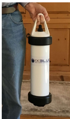
Figure 3 – Acoustic Release iXBlue Oceano 500
